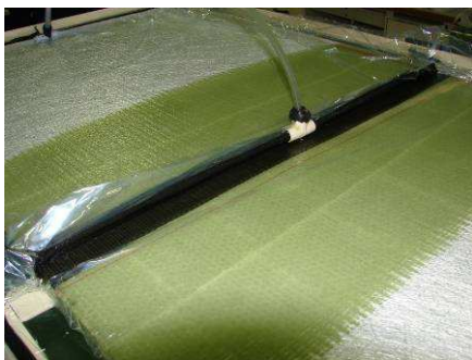
Drainage on the vacuum bag side
